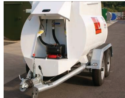
Cabinet with diesel engined pump
