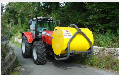
TANK CAN BE LIFTED AND MOVED EASILY BY ANY MACHINE WITH 3 POINT LINKAGE
